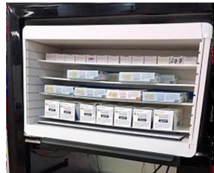
Prototype module to retrofit a refrigerated pharmaceuticals dispensing cabinet with an rfidCollect system
